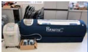
**Fig. 1** The portable hyperbaric chamber (Respiro 270, Oxyhealth) at Hong Kong Sport Institute was used in this study. The maximum chamber pressure was 1.27 ATA. 80-85% O<sub>2</sub> oxygen was delivered to the subject via a standard gas mask for higher efficiency.
