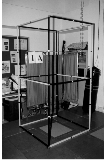
Figure 3. A two-metre high frame was employed for 3-D motion analysis calibration.
