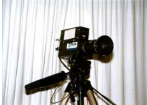
Figure 1. The Peak high-speed video camera was placed at a distance of 5 metres from the subject.
